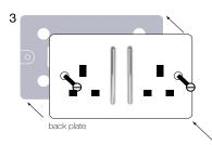
screw back plate onto wall box **NB** do not over tighten as this can distort the plate
